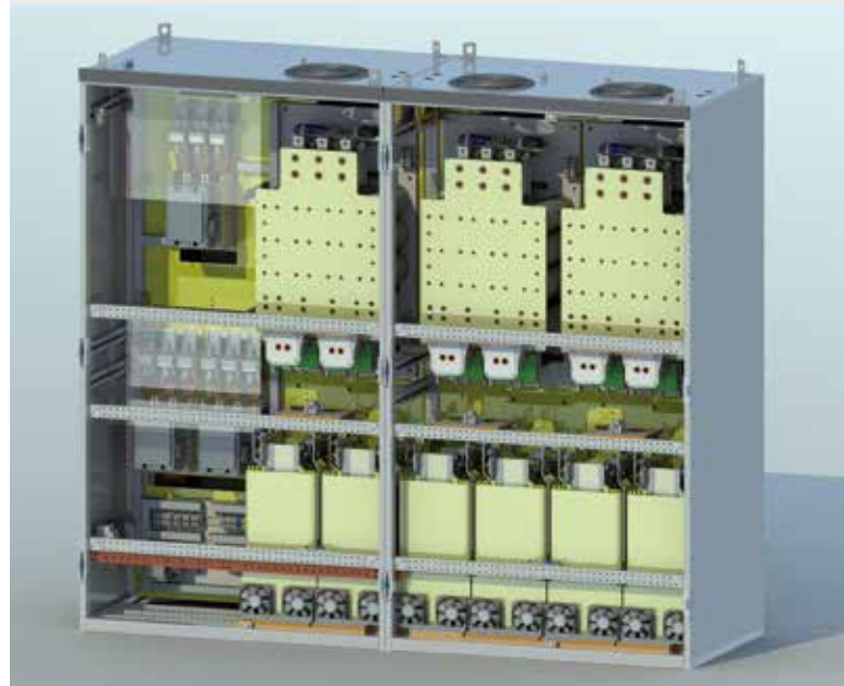
3D design of a 3-phase converter with sine filter for 1300 kVA system output
